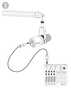
Remark: When the microphone is connected to a mixer or sound card with XLR, the touch control panel on the microphone will not be activated.
